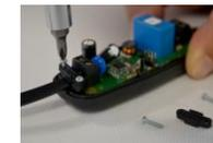
7. Replace the upper shell cover of the switch and tighten with the Phillips screwdriver the assembly screw which joins the two shell covers of the switch
