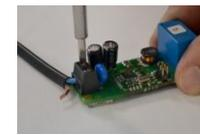
**WARNING: If you reverse the mounting direction of the wires, your SwiidInter™ will not work at all. This will not damage your SwiidInter™, but you will need to reinstall the wires all over again always taking care to disconnect the electrical power cord.**
