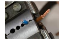
5. Using the flat screwdriver, connect the wires by screwing them into two terminals inside the SwiidInter™ **respecting the directions of the wires** : front towards the device (lamp - near the "L" "N" marking) and back towards the mains (socket - near the light bulb symbol marking)
