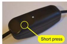
3. The inclusion/exclusion process should then start automatically and the **red LED** will blink before staying lit permanently for 2 seconds. This indicates that the Z-Wave® inclusion/exclusion process was successful
