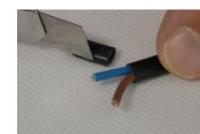
4. With the wire stripper, strip 3-4 mm of the insulation of the two inner wires on both ends
