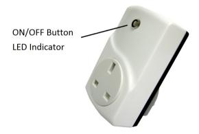
The device is able to switch and measure any electric load up to 400 W. Any load above 400 W is considered as overloading. When overloading is detected the device will turn off the load, lock the local button and indicate the status by flashing the LED for 30 sec. Unplugging and replugging the module will reset the module to normal state. The electrical load can be switched using wireless commands and operating the local button. The LED inside the local button will indicate the dimming status.
